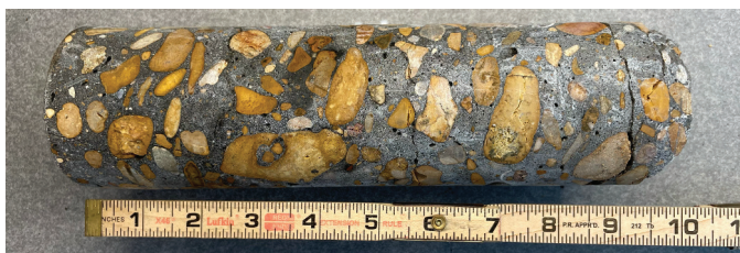
Fig. 8: Core taken from the southwest face of Pier 30
